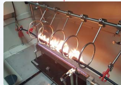
Fire resistance tester BS 6387 IEC 60331
