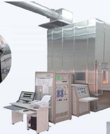
CPR Tester BS 50399 IEC 60332-3-10 IEC 60332-3-22
