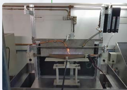
Fire resistance tester with water, shock BS 6387 BS 8491 F30/60/120 BS 50200 BS 7846
