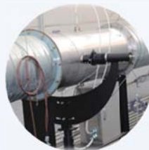
CPR Tester BS 50399 IEC 60332-3-10 IEC 60332-3-22
