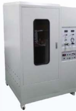
Fire Resistance Tester IEC 60332-1
