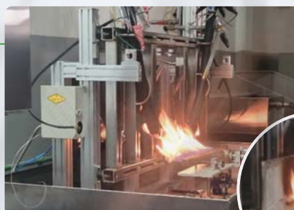
Fire resistance tester BS 6387 IEC 60331
