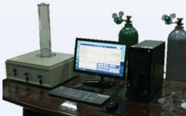
Oxygen Index Tester ISO 4589-2
